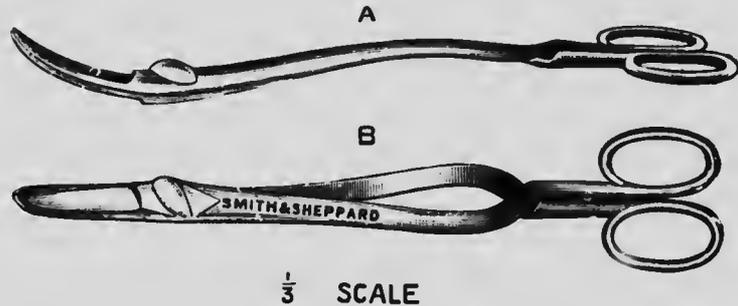
FIG. 201.—Long-handled scissors with double curve.
