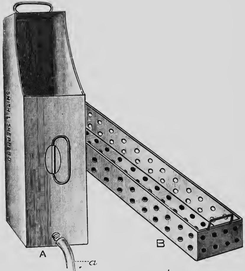
FIG. 78.—Sharpe's steriliser, ready for use as a douche can. A, Douche can. a, Rubber tube. B, Perforated instrument tray.
