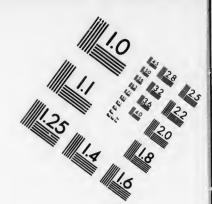
IMAGE EVALUATION TEST TARGET (MT-3)
