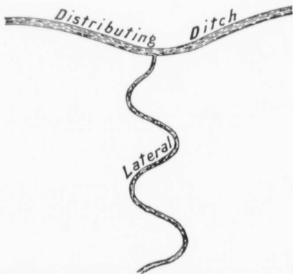
Fig. 17 - Ditch running down steep slope
