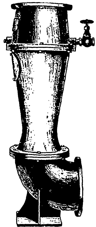
FIG. 3 — UPRIGHT COMBINED AIR INJECTOR AND EXHAUSTER
