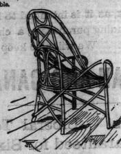
A HOOP POLE CHAIR. This chair can be easily made by any one the can command a supply of smooth hickwho can command a supply of smooth hick-ory saplings. The arrangement of the frame is sufficiently shown in the cut. The sap-lings, where they cross one another, are fastened by nails. The seat is made of small sticks of the same material, the larger por-tions of the saplings being used for the legs. A chair of this kind costs nothing but the
