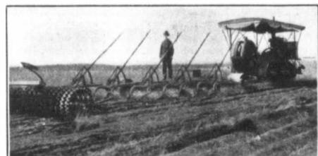
60-H. P. Holt Caterpillar Gas Tractor breaking at Namaka Farm, Namaka, Alberta, Canada. Pulling 10 14-inch engine gang and packer.
