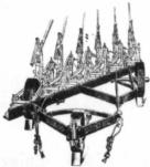
Fig. 12.—Frame of six furrow Mogul Gang Plow.
