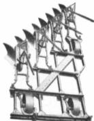
Fig. 5.—Steel frame of John Deere Engine gang.
