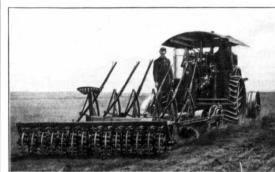
Here a 60 B. H. P. is breaking ground for flax. Note pulverized condition of newly broken ground.
