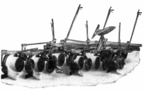
Fig. 26.—Rear view of six bottom plow showing one bottom turned back for travelling on the road, and another lifted up showing amount of vertical movement.
