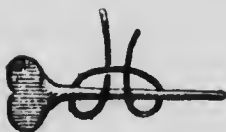
Fig 29—Loops for taking frame keys.
