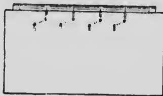
Fig. 58—English style of lacing boards.
