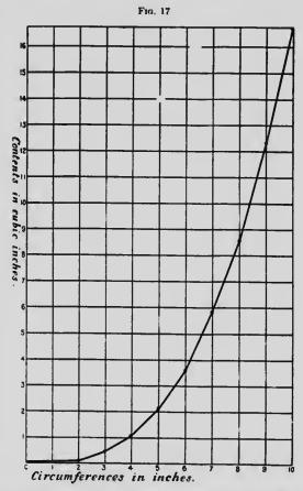
Curve representing the relationship between the circumference of a sphere and its volume, with successive unit increments of circumference. Ordinate—volume in cubic inches. Abscissa—circumference in inches.
