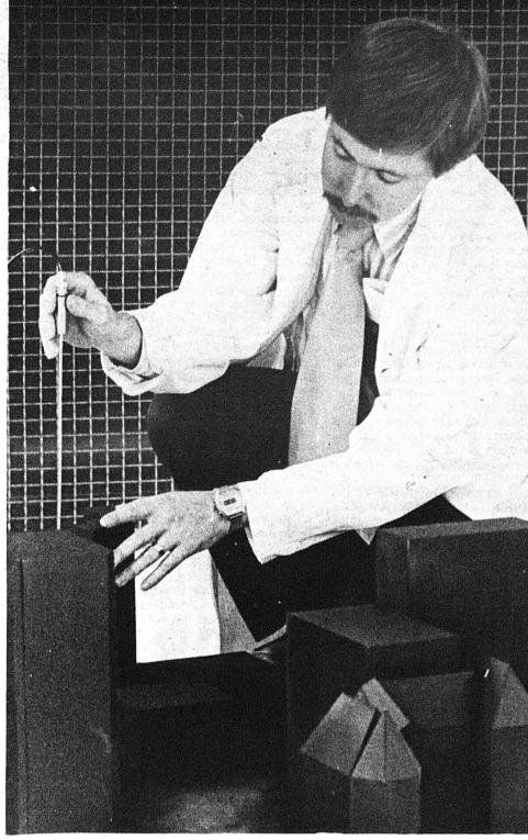
In the main test chamber of the low-speed wind tunnel, Dr. David Wilson measures the intensity of small wind currents in a mock-up of downtown Edmonton. The sensitive prove provides localized measurements which have helped to evaluate wind problems specific to buildings in the MacCauley Plaza are.
