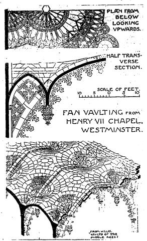
Fan Vaulting in Henry VII.'s Chapel—The Most Intricate Piece of Work Ever Carried Out in Masonry and a Perfect Example of Technical Skill. The Elaborate Construction is Shown Cleverly in the Illustration. The Main Arches Have Voussoirs 3 Ft. 6 Ins. Deep, and the Pendants Which Form Part of the Arch are About 16 Ft. Deep and 5 Ft. Wide. The Small Side Arch Serves by its Connection With the Wall, to Weight and Stiffen the Arch Where it Would be Most Required, that is, Towards the Springing.
