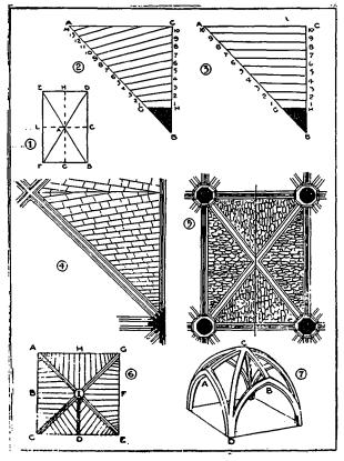
Details of Vault Construction (From Bond's "Gothic Architecture")—2 and 3 Show Respectively the English and French Methods of Stone Filling Between the Vault Ribs. 4—A Vault at St. Saviour's, Southwark. Note the Irregular Stone Jointing at the Ridge, Which Originated the Use of Ridge Ribs in English Work.
