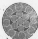
Locked Coil Aerial Cable or Colliery Guide.
