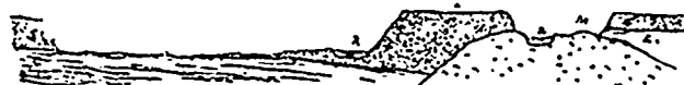
Gorrie Section after the slide. Letters S, G, L, R, M and D have same signification as above given. R, with dot after it, is the former bed of the river, now filled by soil.
