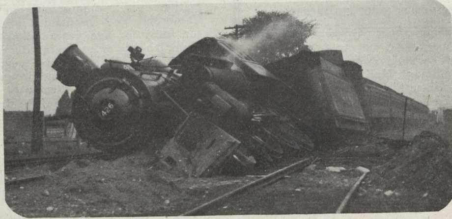
What happens when some hoodlums interfere with a switch "point." This particular accident happened to the North Bay train while entering Toronto.
