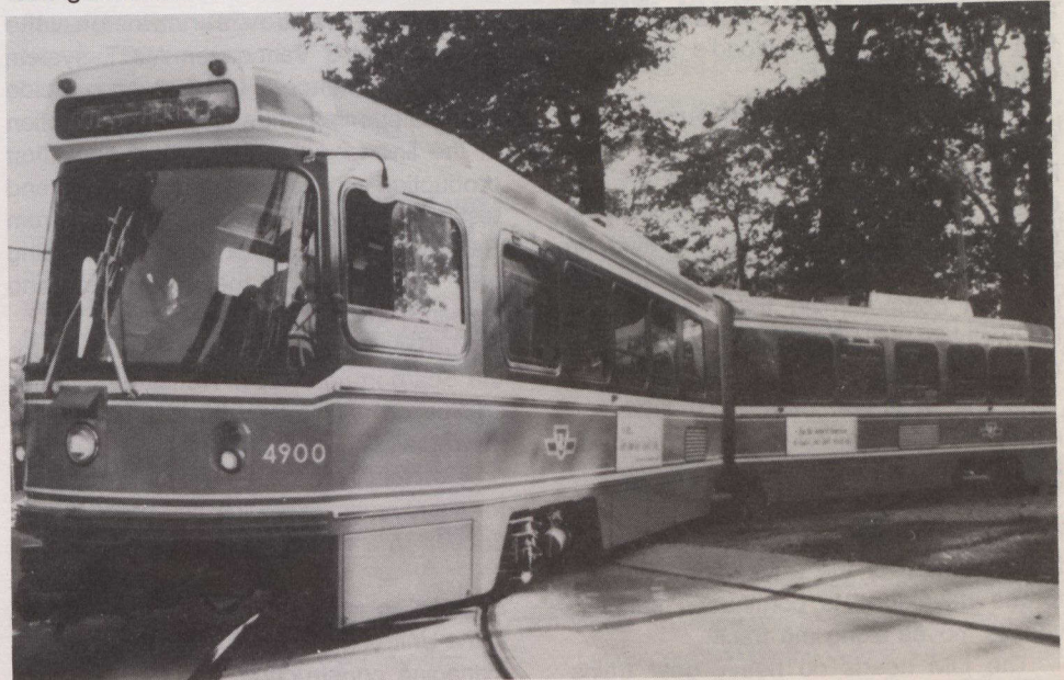
The Articulated Light Rail Vehicle developed by UTDC is capable of doubling passenger loading.
