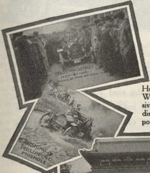
Hupmobile Long-Stroke "32" Touring Car—$1,000. F.O.B. Windsor, including equipment of windshields, gas lamps and generator, oil lamps, tools and horn. Three speeds forward and reverse; sliding gears. Four cylinder motor 3 1/2-inch bore x 5 1/2-inch stroke. Bosch magneto, 106-inch wheel-base, 32 x 3 1/2-inch tires, Color—Standard Hupmobile blue.
