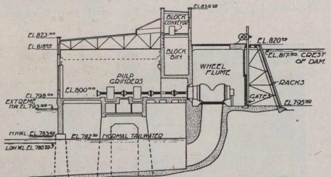
Fig. 8.—Cross-section Through Grinder Room.
