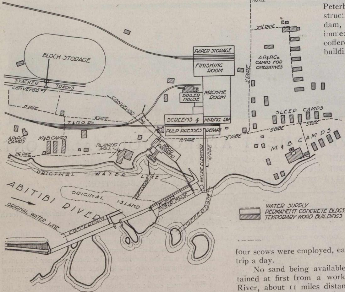
Fig. 3.—General Layout of the Abitibi Power and Paper Company's Development at Iroquois Falls, Ont., Showing also the Construction Camp Arrangement and the Location of Cofferdams for the Construction of the Power House and Dam.
