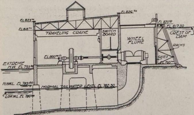
Fig. 6.—Cross-section Through Generator Room.
