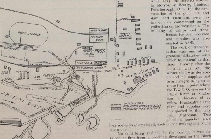
Fig. 3.-General Layout of the Abitibi Power and Paper Company's Development at Iroquois Falls, Ont., Showing also the Construction Camp Arrangement and the Location of Cofferdams for the Construction of the Power House and Dam.
