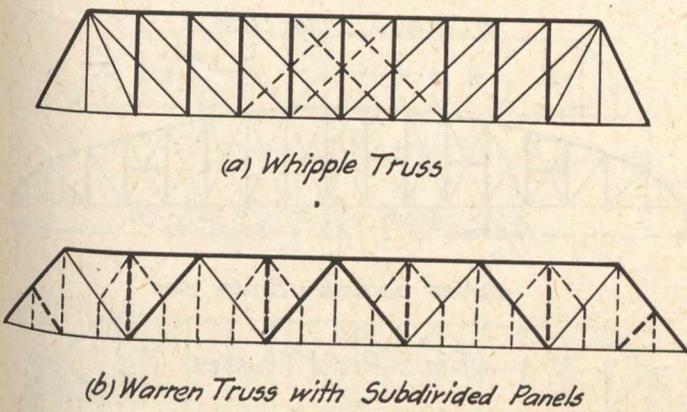
Fig. 1 - The Whipple Truss and its Successor
