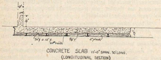
CONCRETE SLAB 11'-0" SPAN, 30' LONG.
