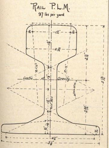
We expect the combination of a 100-pound rail held by nail spikes to soft ties in a poor gravel ballast to carry twice the load at the same speed with the same safety that is attained in Europe with the same rail held by screw spikes to harder ties in generally a stone ballast and in much better conditions of temperature.
