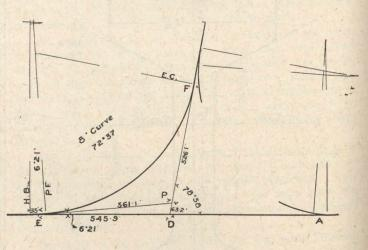
Let its total angle be known as  $I_3$ .  $I_3 = 180 - I.$   $= 180^\circ - 101^\circ 02'.$   $= 78^\circ 58'.$ Let angle of long curve be  $I_4$ . Then  $I_4 = I_3 - F.$
