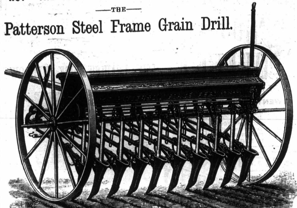
It possesses every desirable quality arranged in the most simple and attractive form. Has a positive force feed which does not clog or crack the grain. It commences to sow as soon as the horses move, misses no ground, covers the seed perfectly, and the depth can be instantly regulated as required. Sows ALL GRAINS from FLAX SEED TO PEAS AND BEANS with accuracy and uniformity. Has a refined Channel Steel Frame and our New Patent Hoe Connection; the strongest, simplest and best yet invented.
