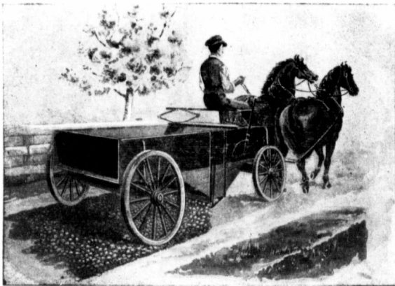
New Style Stone and Gravel Spreading Waggon.
