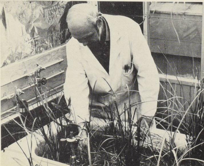
into a grid system based on squares 500 feet to the side. This system provides a basis for systematically locating sampling sites. Sampling will continue the year round at selected sites with others being added as required by seasonal changes. At each site, the water and suspended matter, the sediment and plant and animal life are analysed to establish the pollutant level associated with each compartment.
