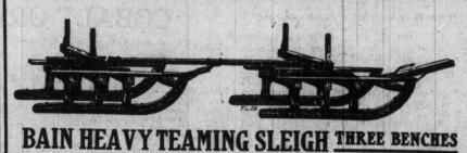
ESPECIALLY ADAPTED FOR TEAMSTERS' USE. TRACK, 3 FEET FROM CENTRE TO CENTRE OF RUNNERS. HEIGHT, TO TOP OF BOLSTER, 19 INCHES. SHOES: 2 OR 2 1-2-INCH FACE.
