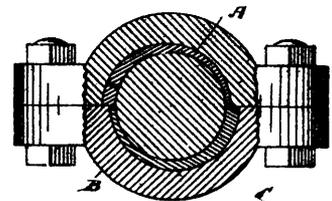
37402 Irvin's Fastening for Securing a Pulley to a Shaft.
