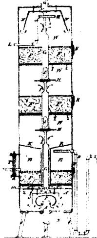
37336 Austin's Combined Feed Water Heater, Filter and Condenser, and Lime and Grease Extractor.
