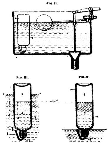
37399 Taylor's Apparatus for Automatically Supplying Disinfectant Liquids to Closets, etc.
