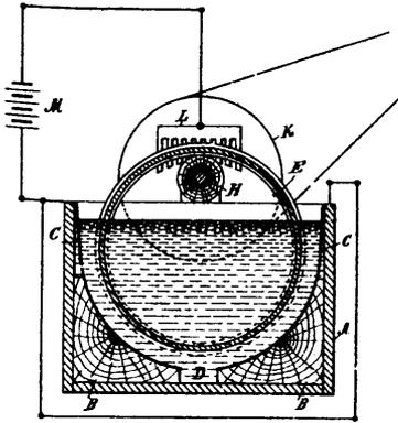
37341 Farmer's Apparatus for Producing Sheets of Metal by Electro-Deposition.
