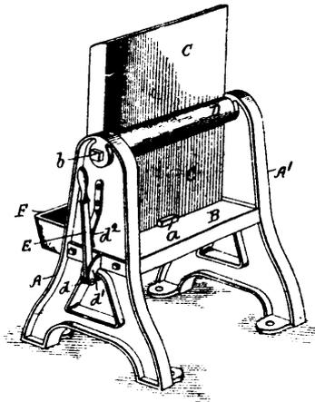
37345 Covel's Device for Hammering and Straightening Saws.
