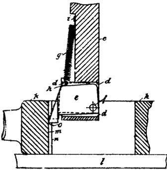
37382 Carter's Tool Holder and Cutting Tools for use in Slotting Key Ways in Pulleys, etc.
