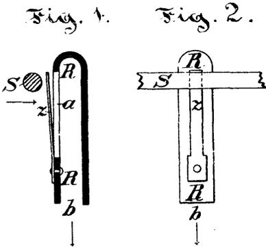
37332 Gumbel's Mechanism for Striking Strings by means of Reeds Moved by Air:
