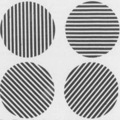
Test Figures for Detecting the Presence of Astigmatism.
