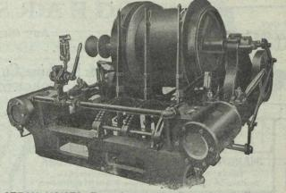
STEAM HOISTS, Reversing or Non-Reversing, 2 Types— Drums Friction Driven, or keyed to shaft. Operating Levers, Piping, etc., arranged to suit the buyer.
