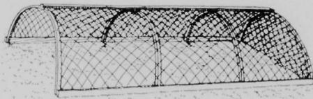
Take four old carriage rims and fasten them together 4 feet apart, by three 1 by 2-inch strips, 12 feet long. Two strips are nailed at each end of the rims near the ground, and the other at the top. Place your wire over the rims and cut it the right length, so as to have just enough to tack on the strips. I use 1-inch mesh wire netting 6 feet wide and 14 feet long—the extra 2 feet to close up one end. I place a coop of hen and chicks at the front or open end.
