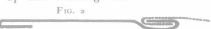
FIG. 2 Fig. 2 shows the side locks. Note the deep firm grip which allows ample room for expansion and
