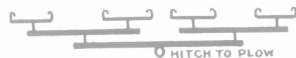
No. 3.—Four-horse Evener, for use when horses are hitched abreast on Harrows, etc.
