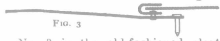
FIG. 3 No. 3 is the old-fashioned cleat shingle now almost entirely driven from the market by the Safe Lock. These do not always shed water, and it is almost impossible to keep them from leaking after they have been on for a season or two.
