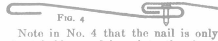
FIG. 4 Note in No. 4 that the nail is only about half way driven into the sheeting, leaving a large surface exposed to the weather. This makes a very insecure fastening for a roof, and this is still further weakened by the springiness of the steel, which has a tendency to pull out the nails, causing a loose, leaky, rattling roof.
