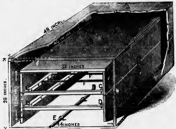
FIGURE 2. INTERIOR OF INCUBATOR.
