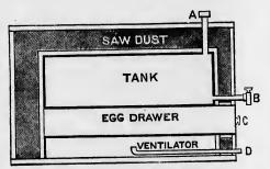
FIG. 6. SECTIONAL VIEW OF INCUBATOR.
