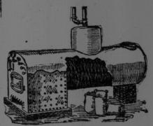
This is composed of 90% Asbestos fibre, and a cementing compound forming a light, porous covering, partaking of the nature of a felt and a cement, to be applied with a trowel to Steam Pipes, Boilers, etc., while heated. This is recommended for all steam heated surfaces. Furnished dry, to be mixed with water to the consistency of mortar, and can easily be applied by unskilled workmen.
