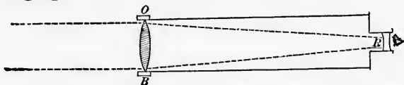
FIG. 28.—The Galilean telescope. The dotted lines show the course of the rays through the lenses.
