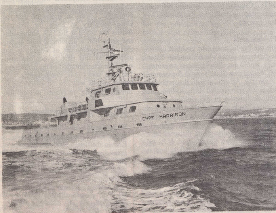
The Cape Harrison, one of the latest additions to the fisheries patrol fleet, ensures that Canada's fishing laws are observed off the coast of Newfoundland. The 120-foot aluminum vessel is capable of speeds of over 20 knots.
