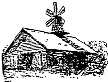
SIX-FAN HOLLAND WINDMILL, designed and built by Henry Dorman, near Portal, Neb. Diameter nearly 20 ft. Runs a 6-horse feed grinder. Cost $50.
