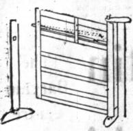
strikes the nail in (b) the gate will begin to raise out of the slot at (d), which is about two inches deep. (e) is an old post sunk in the ground flush with the surface. The heel of the gate turns in an auger-hole in (e). Wagongrease keeps water from freezing in this hole. (d) should be three by six by twenty-four inches, and spiked to the post. One or more barbed-wires should be used on all farm gates. The dong bar of the latch should be about three feet or longer.
