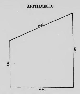
38. The above figure represents the end of a shed 20 ft. long, and other dimensions as shown. Find the number of feet of inch lumber required to enclose it.
