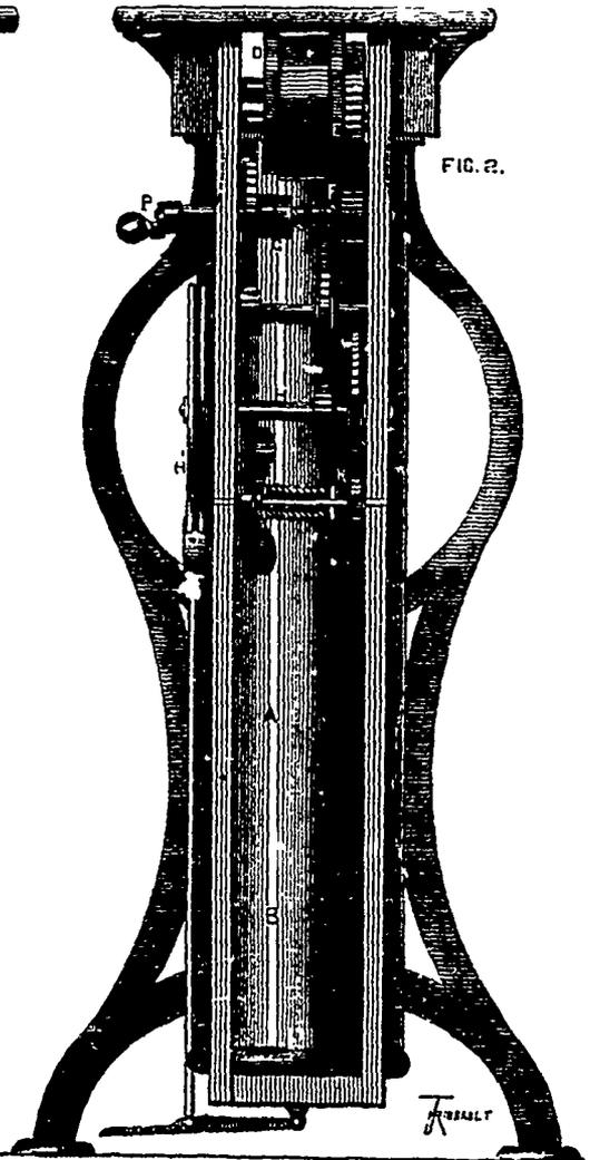
APPARATUS FOR DRIVING SEWING MACHINES.
