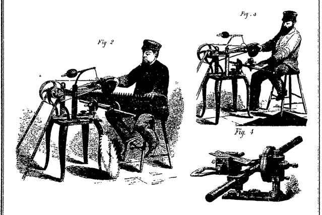
FLEXIBLE SAW AND TOOTH FILING APPARATUS.
