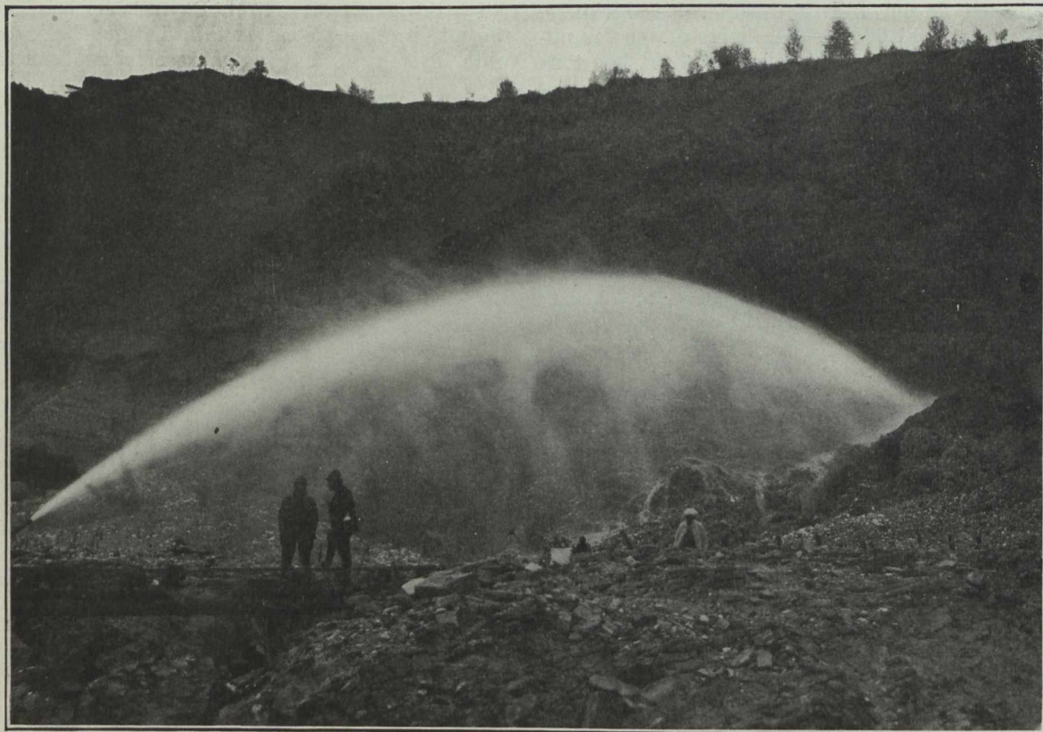
Hydraulic mining the High Level "White Channel" Gravels on Property of the Yukon Gold Co., Bonanza Creek, Klondike
