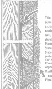
This Cut represents a cross section of wall. showing Plaster-Stucco. Stucco Board (note the Key holding Stucco) Asphalt, Mastle and Fibre Paper
