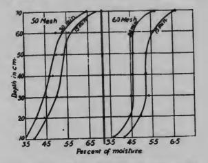
individual points were sometimes decidedly off the curves, but although the experiments were repeated in these cases, no better agreement could be obtained; the accurate determination of small amounts of moisture in these sands proved to be difficult, probably owing to sampling. The average per cent of moisture was determined by measuring the areas under the curve, and dividing this by the height which gave the width of the rectangle of equal area.
