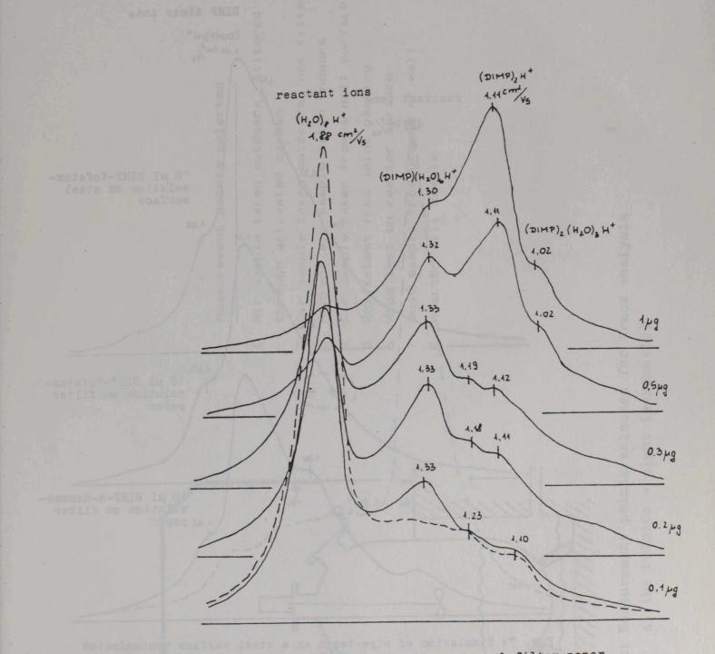
Fig. 6: Spectra of DIMP applied on aerosol filter paper, for different contents of DIMP
