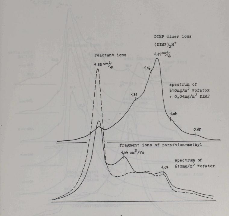
Fig. 2: Influence of 610mg/m<sup>3</sup> Wofatox on the shape of the spectrum of 0,04mg/m<sup>3</sup> DIMP
