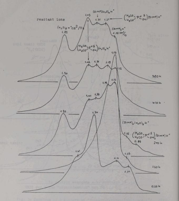
Fig. 5: Spectra recorded from a rubber sample contaminated with Wofatox +  $1^{\circ}/_{\circ\circ}$  DIMP mixture, with increasing storage time
