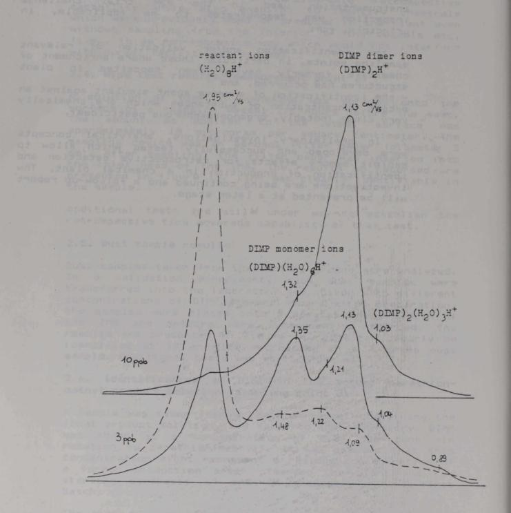
Fig. 1: IMS spectra recorded for 3 and 10 ppb DIMP in air
