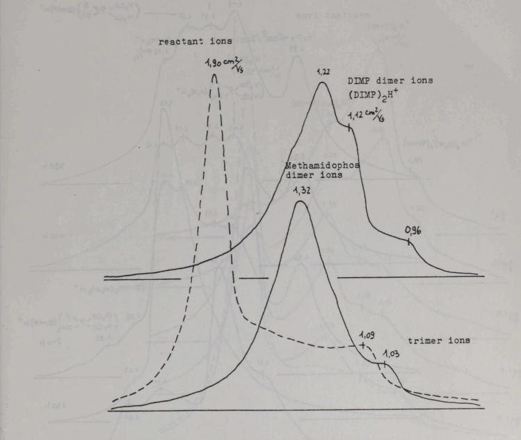
Fig. 4: Spectrum of a gasphase mixture of 10 ... 20 ppm "Methamidophos" and 5 ppb DIMP
