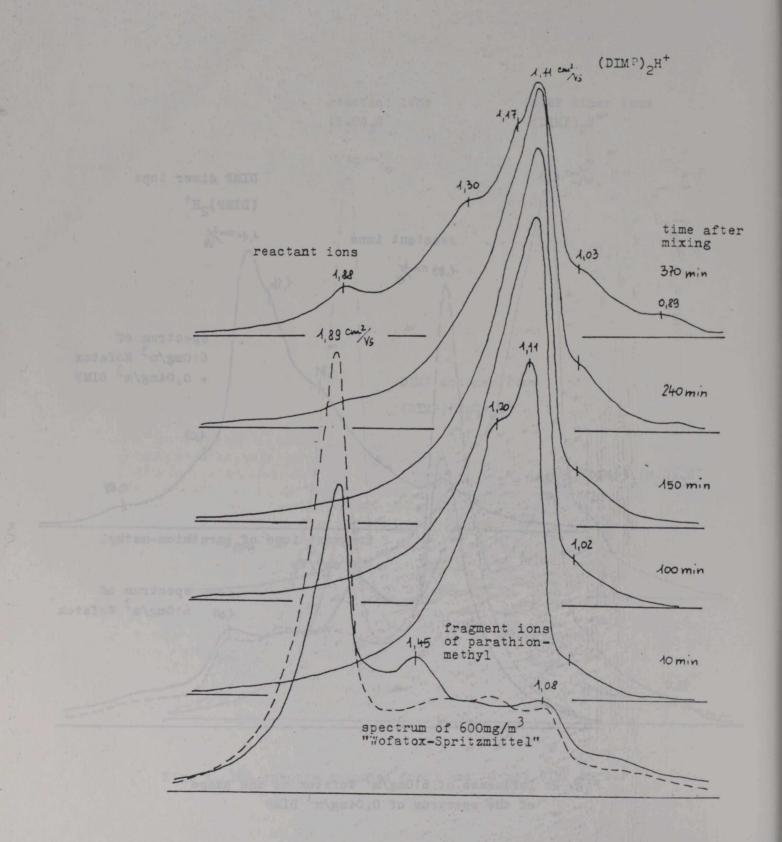
Fig. 3: Spectrum of a mixture of "Wofatox-Spritzmittel" and  $1^{\circ}/_{\circ\circ}$  DIMP
