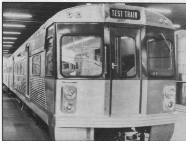
Self-propelled, electric suburban rail cars built for the Delaware River Port Authority, Philadelphia, by Versatile Vickers.
