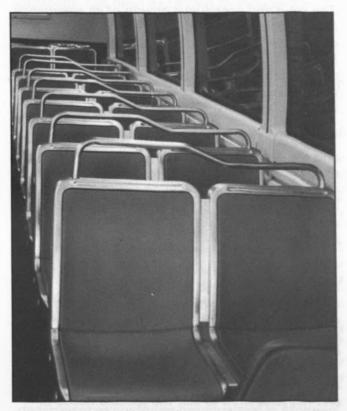
Innovator Model 850, with low maintenance, impervious to graffiti, vandal and fireproof stainless steel shells, with tamperproof padded or hard cushion inserts. In service in Toronto, soon to be in Boston.
