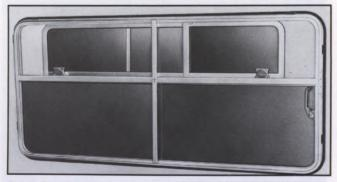
Storm-Tite transit bus window, model MVII, upper slider sash and lower picture window.
