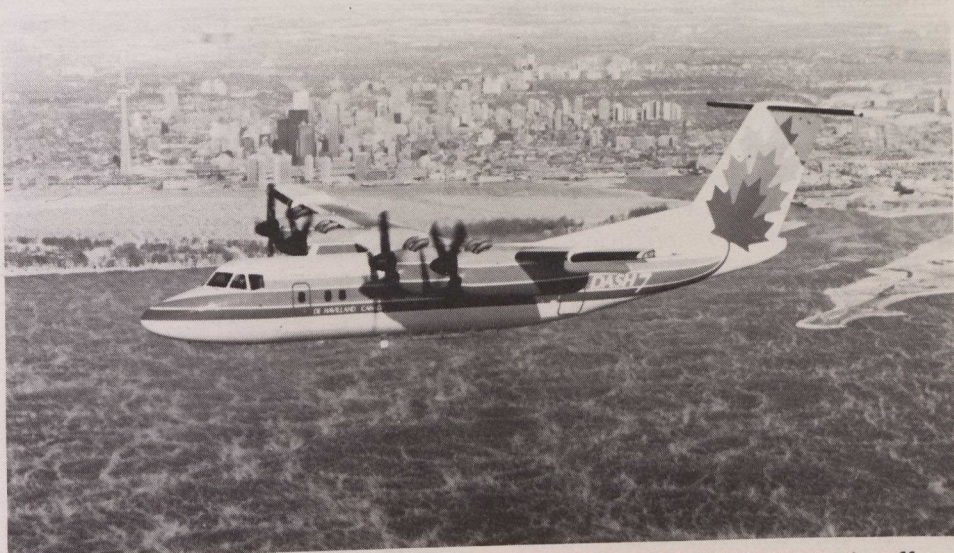
The de Havilland Aircraft of Canada Limited 50-passenger DASH 7 short take-off and landing (STOL) aircraft. To date 86 of these popular short-haul transports have been delivered to customers throughout the world.
