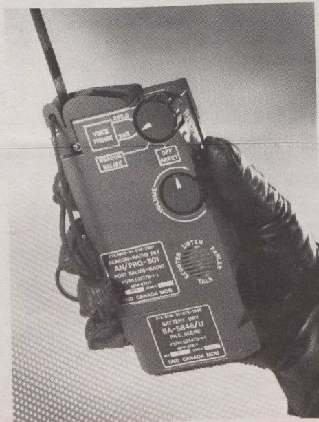
The Garrett Manufacturing Limited personal locator beacon. This light-weight emergency beacon/transceiver provides an emergency homing signal as well as two-way voice communications with search aircraft.
