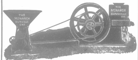
10 in. Grinder and 8 H.-P. Hopper-cooled Engine.
