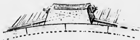
FIG. 8.—Showing clip made of wood or iron to be used where posts are not left in sides.
