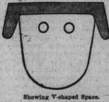
We can supply the tires and new wheels complete—if so desired. We have the Solid Rubber Dunlop Carriage Tires—an entirely new and patented tire which has many points of superiority over A steel flange with a V-shaped space between steel and rubber allows the necessary space for expansion and gives full play to
