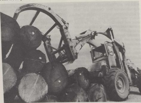
Logs to be processed into veneer are gobbled by a log-loader.
